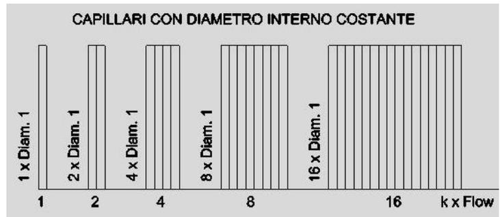
All the equal capillaries that make up a group are arranged in parallel so that the flow corresponding to a group is equal to the sum of the flows carried out by the capillaries of the group itself.
